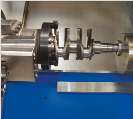
Eccentric collet system for Crank shaft pin turning
