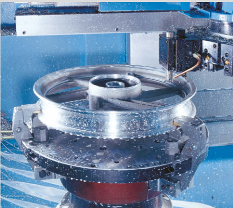
Special face clamping and ID collet for Alloy Wheel
